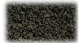
Catalytic media is used for oxidation of metals and H 2 S removal
